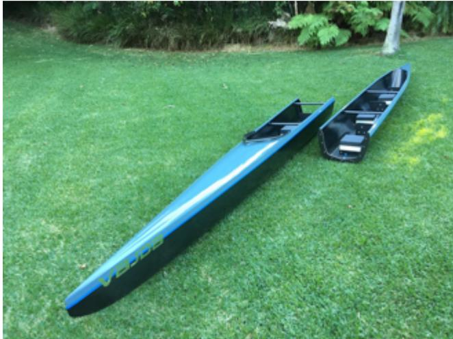
This hi-kneeling C4 was made by Vajda and is the second top build. The top build cost \$15K and so, unusually for me, opted for the next one down (\$10K). It is carbon fibre and is wider and much more stable than the similar C2 that you may have seen me in, or the C1 I usually paddle. I had the C4 made in two halves so that I could transport it on my small car.
